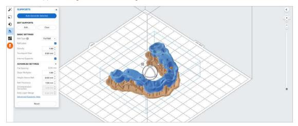
To allow for simple and precise assembly, ensure that there are no supports near the guide sleeve holes or on the intaglio surfaces. Use the manual support editing feature to closely inspect support locations and add or remove supports as needed.
