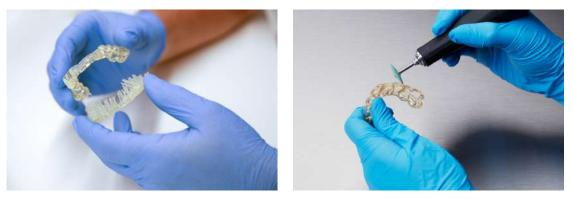
Note: Remove supports only after post-curing to ensure that parts do not warp.
